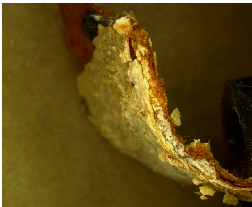
Pictures 1 and 2 – Magnified views of calcium buildup on evaporative pads. Calcium covered pads make an even rougher surface for debris to get caught on and clog pad flutes.
