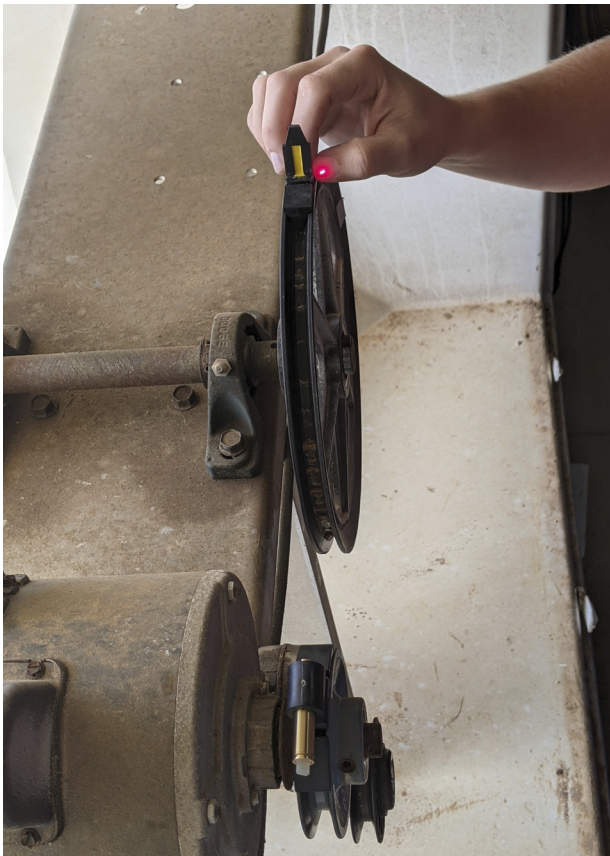
Figure 6: Left photo, the laser method is used on a fan where the pulleys are out of alignment approximately 5/8 inch. Right photo, the laser is hitting inside the yellow acceptable strip, showing the pulleys are in correct alignment.
