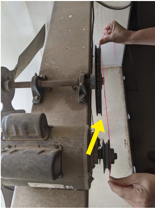
Figure 3: Left, the string method used on a fan where the pulleys are out of alignment approximately 5/8 inch. Right, the string method showing four points of contact and that the pulleys are in correct alignment.
