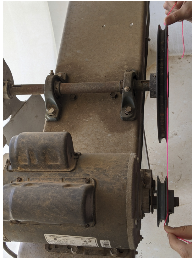
Figure 3: Left, the string method used on a fan where the pulleys are out of alignment approximately 5/8 inch. Right, the string method showing four points of contact and that the pulleys are in correct alignment.
